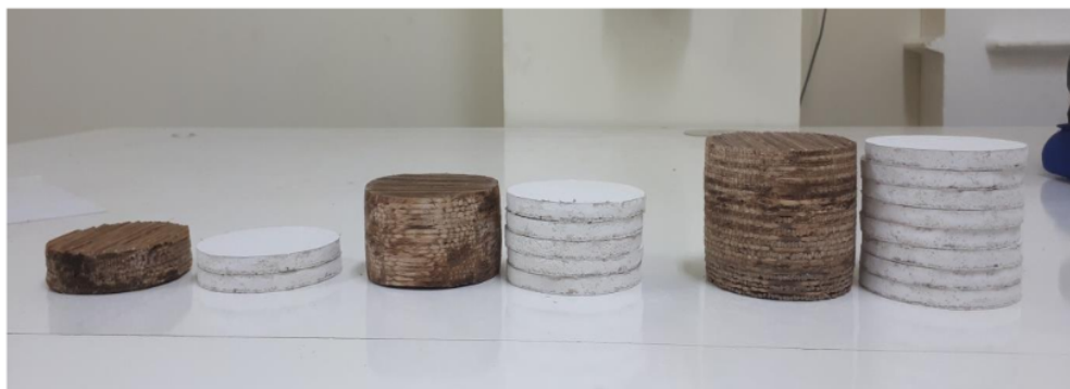
Figure 6. Sample of coconut leaf midribs and acoustical gypsum with variety of thickness and configurations
