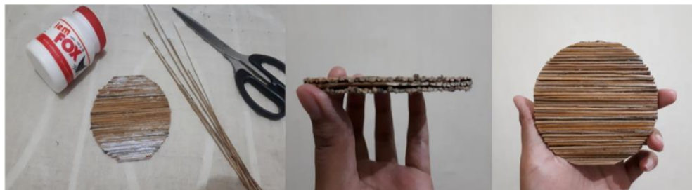
Figure 3. Coconut leaf midribs are glued together one by one using PVAc adhesives
